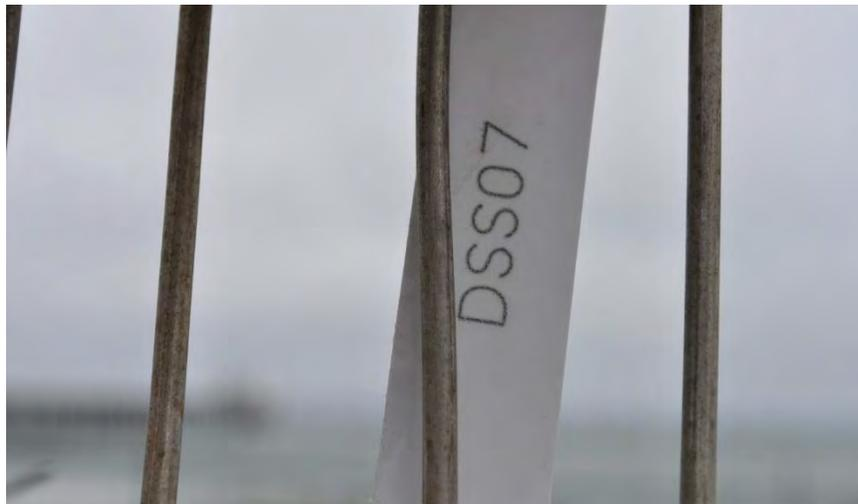
Figure B19. Stainless Steel Wire Coupon
