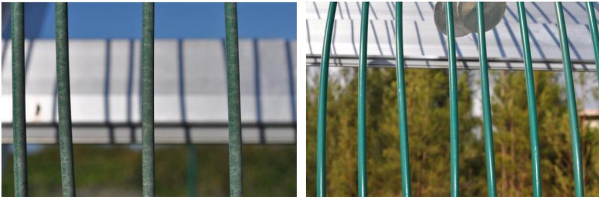
**Figure 19. Aluminum wire coupon at FRF (left) and KTA (right) after 6 months of exposure.**
