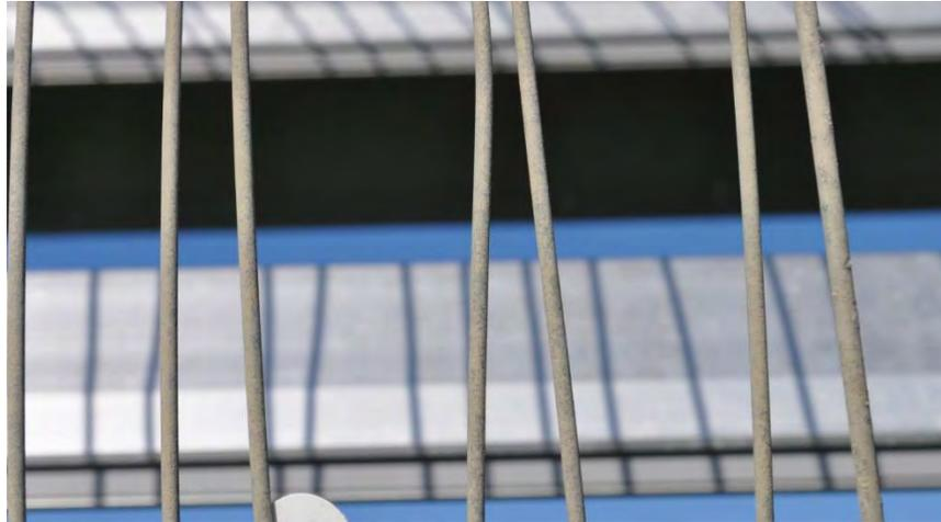
Figure B33. Aluminized Steel Wire Coupon
