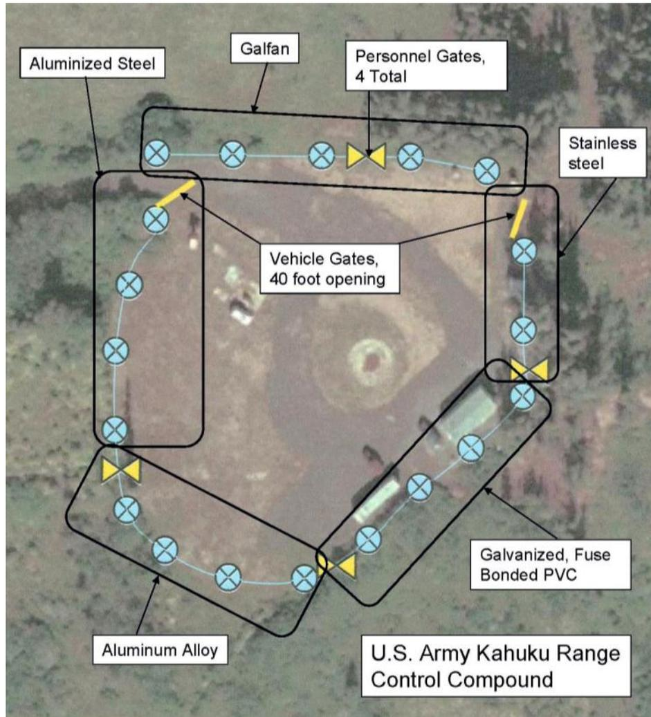
The following four railing materials were installed in 12 ft sections for exposure testing:
