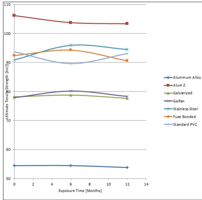
Figure 41. Force calculated from tensile testing of wire coupons exposed at KTA.
