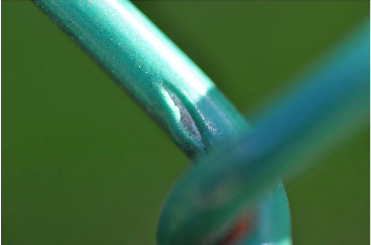
*Figure B129. Fuse Bonded PVC Coated Galvanized Wire Fencing*
