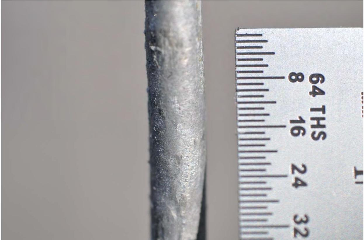
*Figure B166.* Aluminized Steel Wire Coupon
