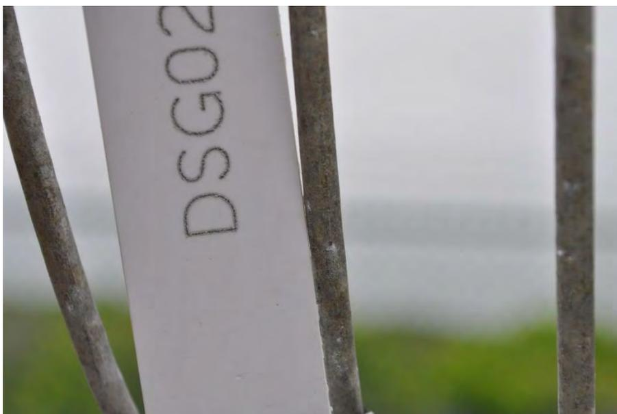
Figure B11. Standard Galvanized Wire Coupon
