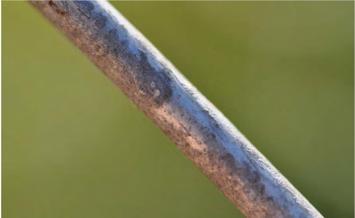
*Figure B127. Aluminized Steel Wire Fencing*
