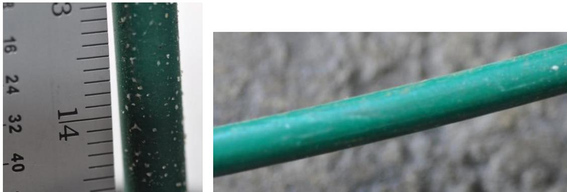
Figure 26. Aluminum wire coupon at the FRF (left) and KTA (right) after 12 months of exposure.
