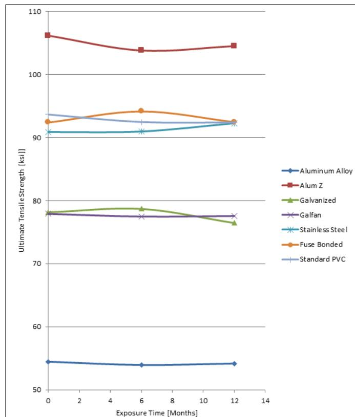
Figure 42. Force calculated from tensile testing of wire coupons exposed at Treat Island.
