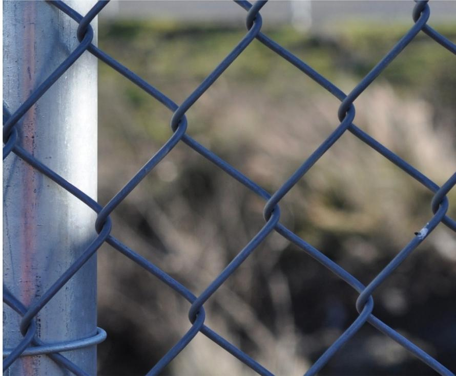
Figure A14. Aluminized after 12 months exposure showing corrosion on less than 5% of the total surface area.
