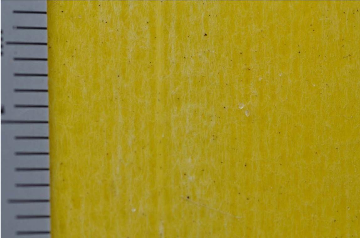
Figure B42. FRP Railing Coupon
