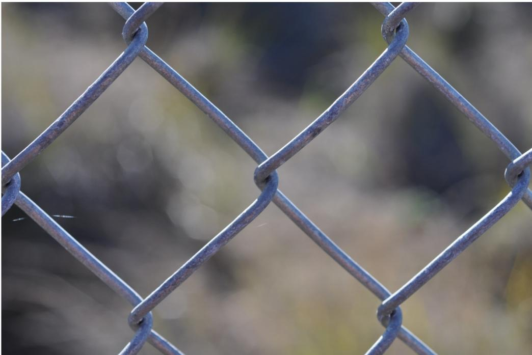
Figure A11. Aluminized after 6 months exposure.
