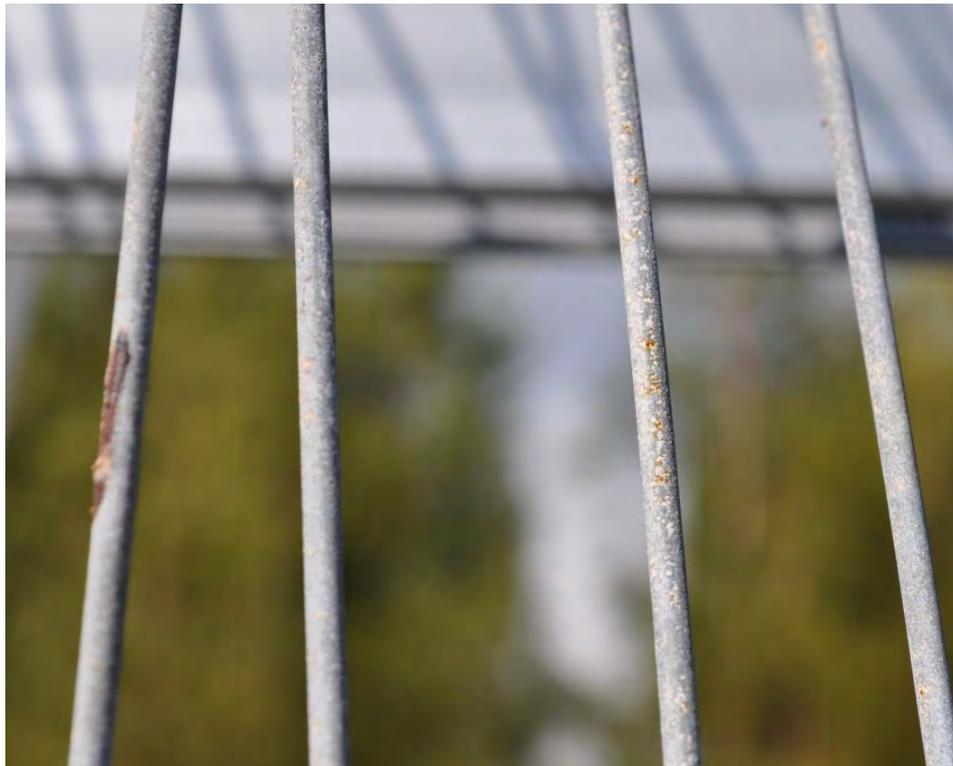
Figure B86. Standard Galvanized Wire Coupon
