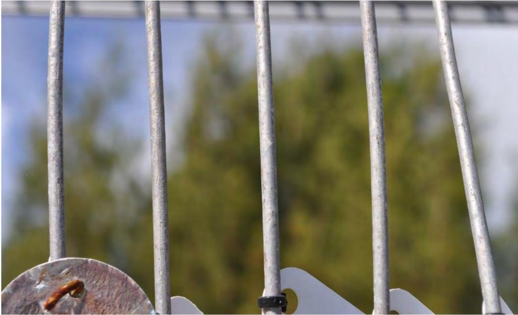
*Figure B88.* Aluminized Steel Wire Coupon
