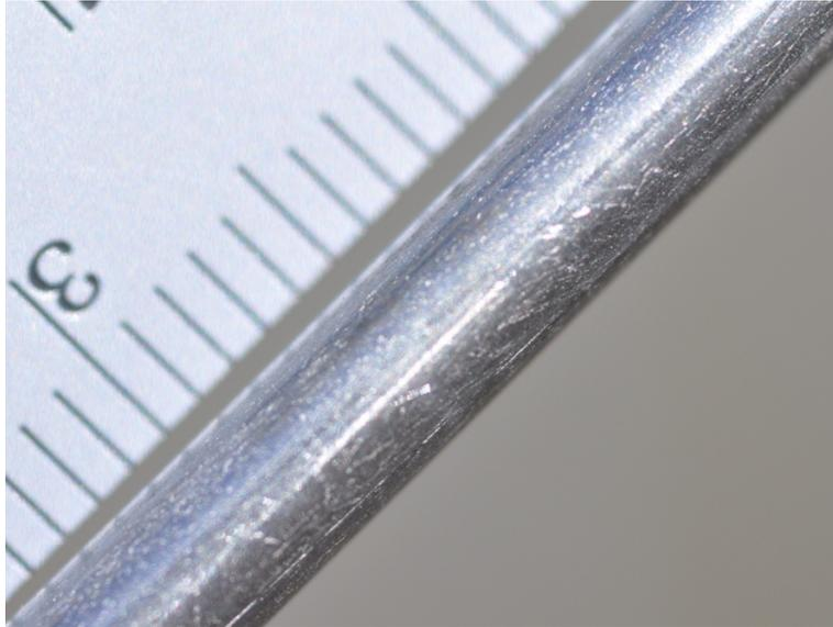
Figure A19. Galvanized after 12 months exposure.
