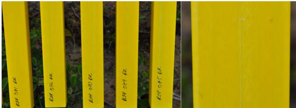
Figure B1. FRP Railing Coupon
