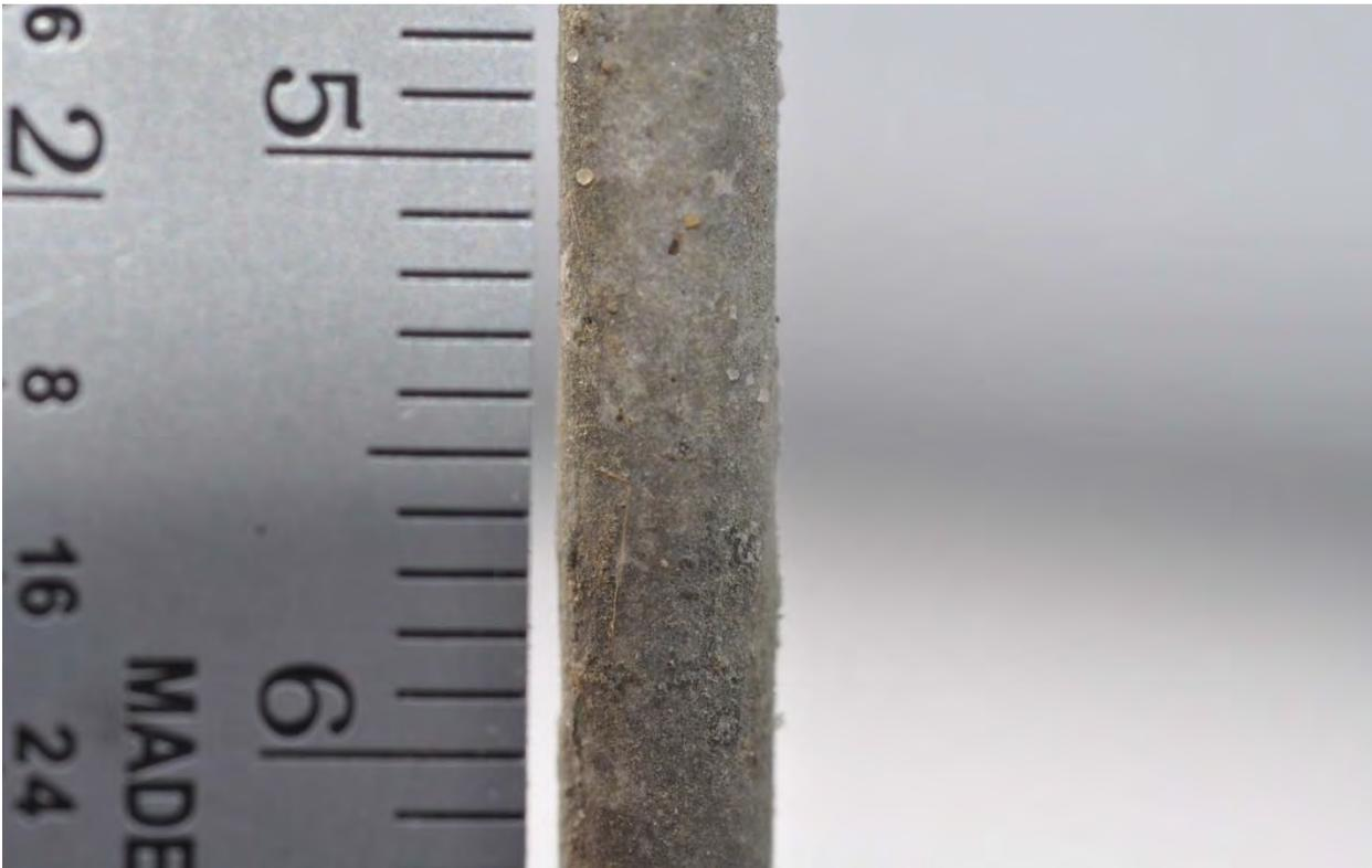
Figure B52. Standard Galvanized Wire Coupon
