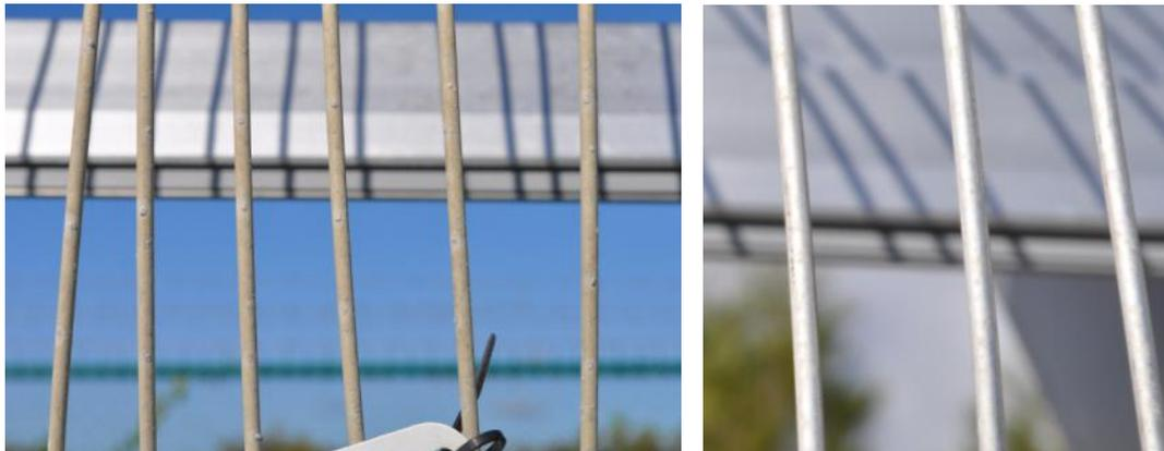
Figure 20. Stainless steel wire coupon at FRF (left) and KTA (right) after 6 months of exposure.
