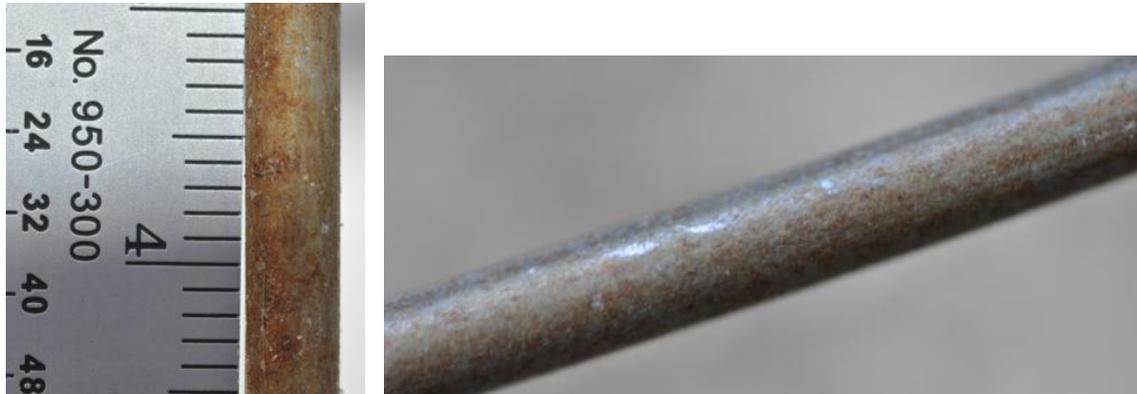
Figure 28. Galvan wire coupon at FRF (left) and KTA (right) after 12 months of exposure.
