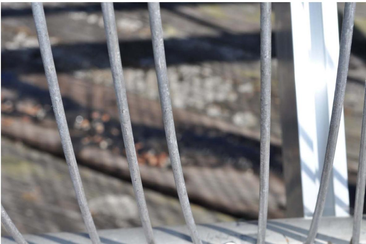
*Figure B143. Aluminized Steel Wire Coupon*
