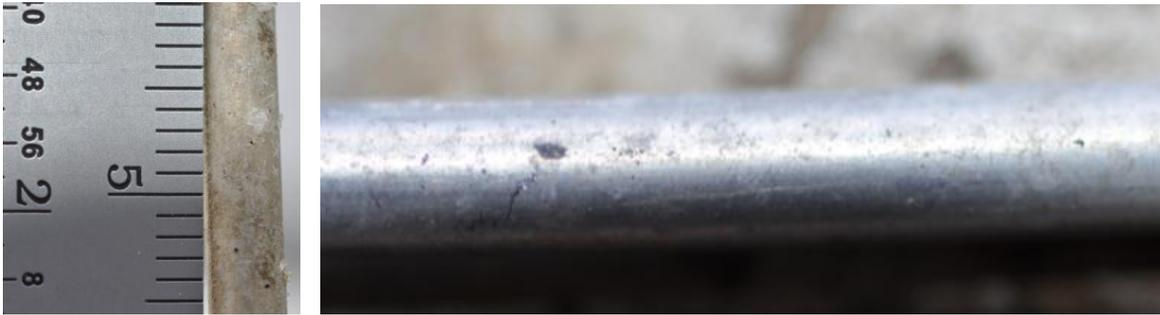
Figure 27. Stainless Steel wire coupon at FRF (left) and KTA (right) after 12 months of exposure.
