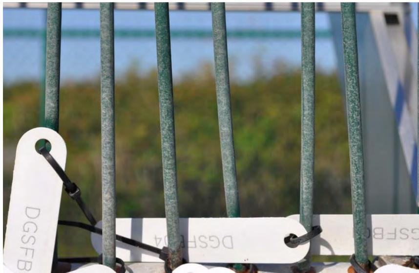
Figure B34. Fuse Bonded PVC Coated Galvanized Wire Coupon
