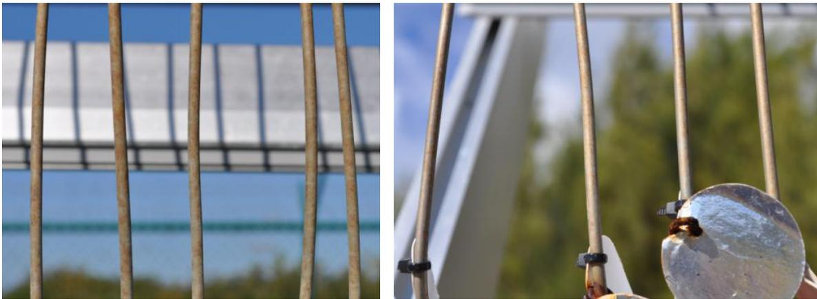
Figure 21. Galvan wire coupon at FRF (left) and KTA (right) after 6 months of exposure
