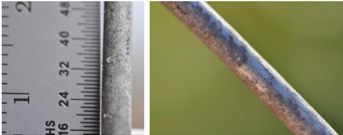
Figure 25. Fuse bonded PVC coated wire coupon at FRF (left) and KTA (right) after 12 months of exposure.
