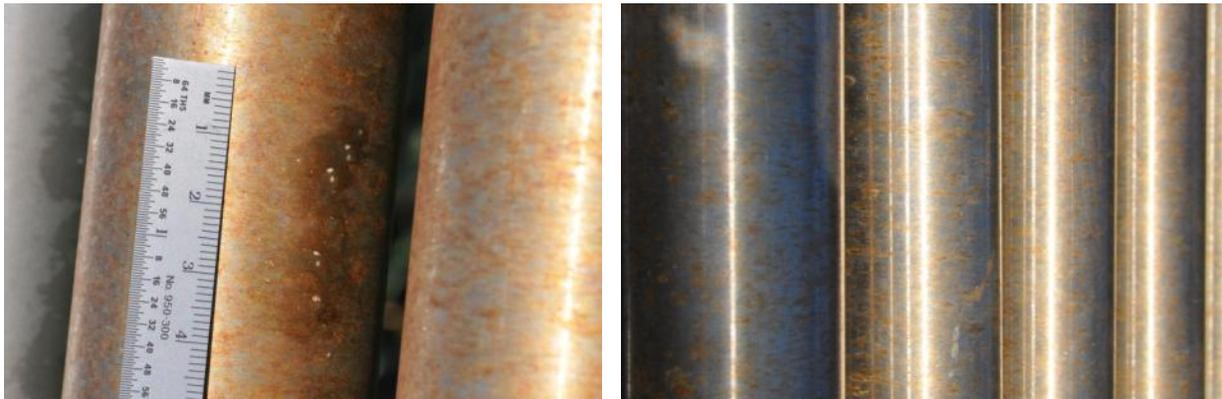
Figure 32. Aluminum railing coupon at FRF (left) and KTA (right) after 6 months of exposure.
