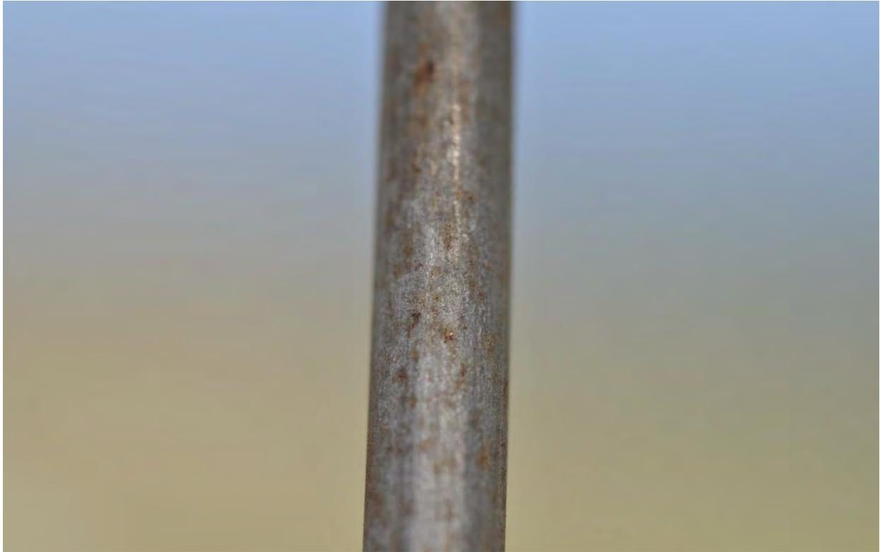
*Figure B114.* Stainless Steel Wire Coupon
