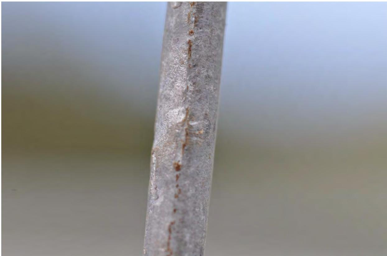
*Figure B107. Aluminized Steel Wire Coupon*
