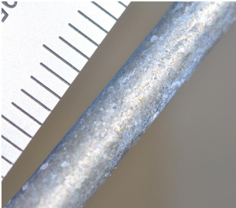
Figure A20. Stainless steel after 12 months exposure.
