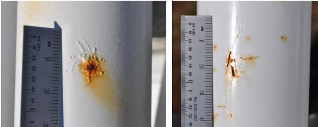
Figure 31. Stainless steel railing coupon at FRF (left) and KTA (right) after 6 months of exposure.
