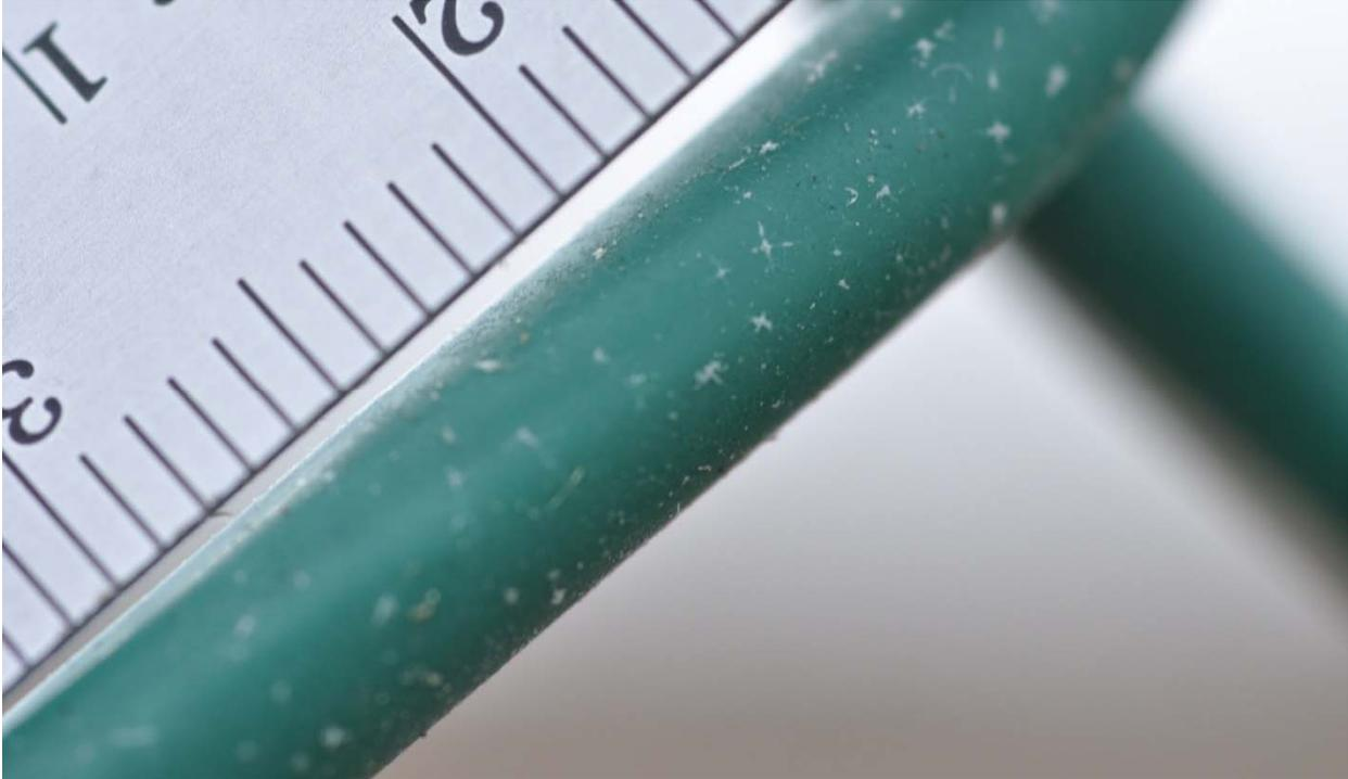
Figure B56. Fuse Bonded PVC Coated Galvanized Wire Fencing
