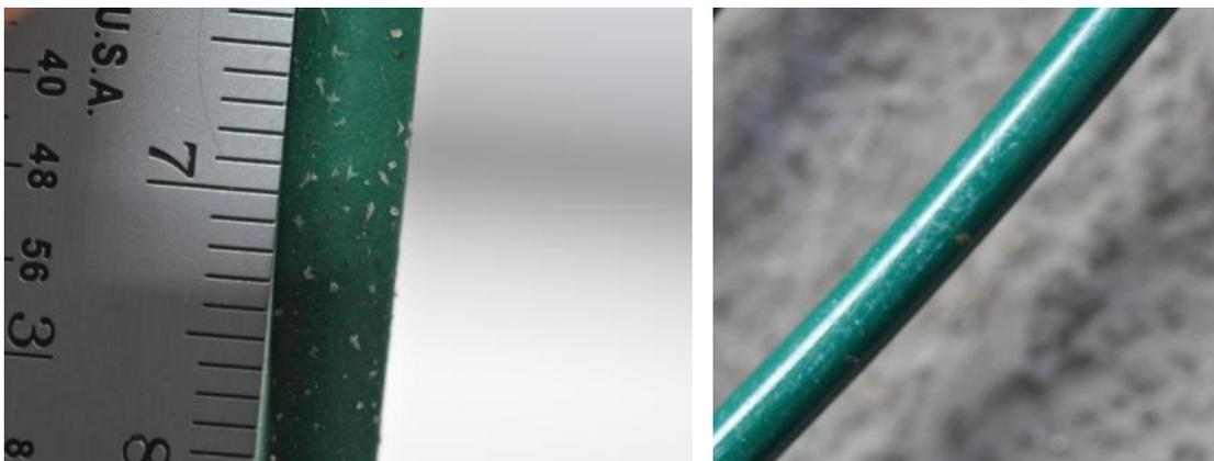
Figure 23. Standard galvanized steel wire coupon at FRF (left) and KTA (right) after 12 months of exposure.
