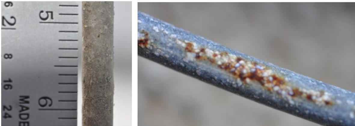
Figure 24. Aluminized steel wire coupon at FRF (left) and KTA (right) after 12 months of exposure.
