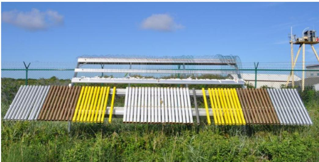
Figure 13. Railing and wire coupons installed on exposure rack placed at 45 degree angle at Treat Island.
