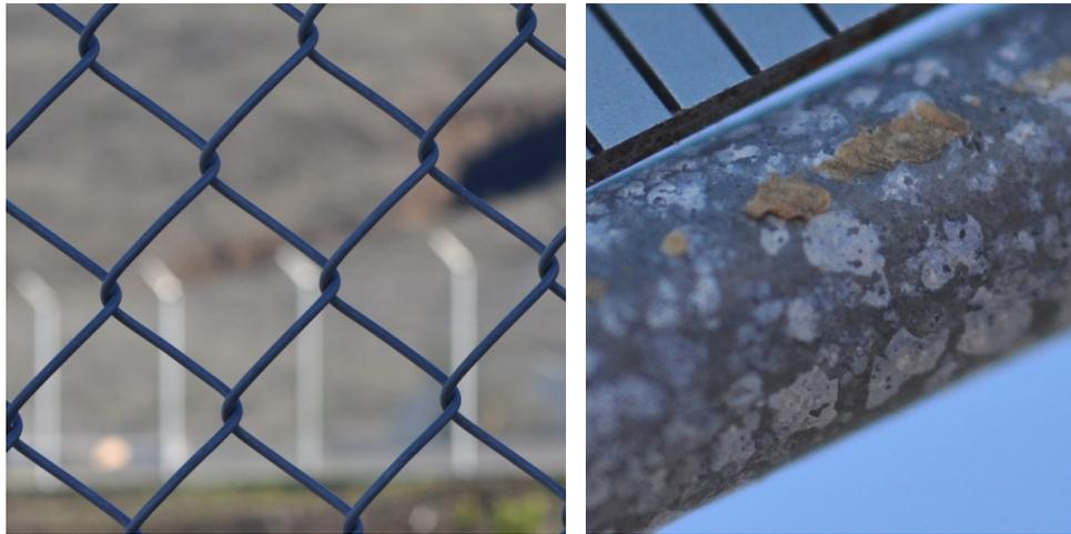
Figure A17. Fuse-bonded PVC undamaged (left) and damaged (right) after 12 months exposure.
