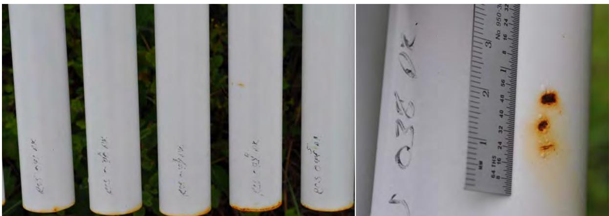
Figure B3. Coated Steel Coupon
