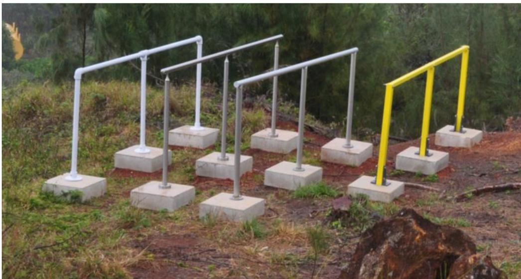
Figure 8. Railing test sections installed at the FRF.
