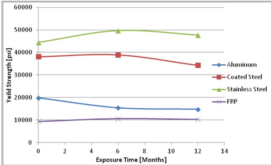
Figure 44. Yield stress calculated from flexure testing of railing coupons exposed at KTA.
