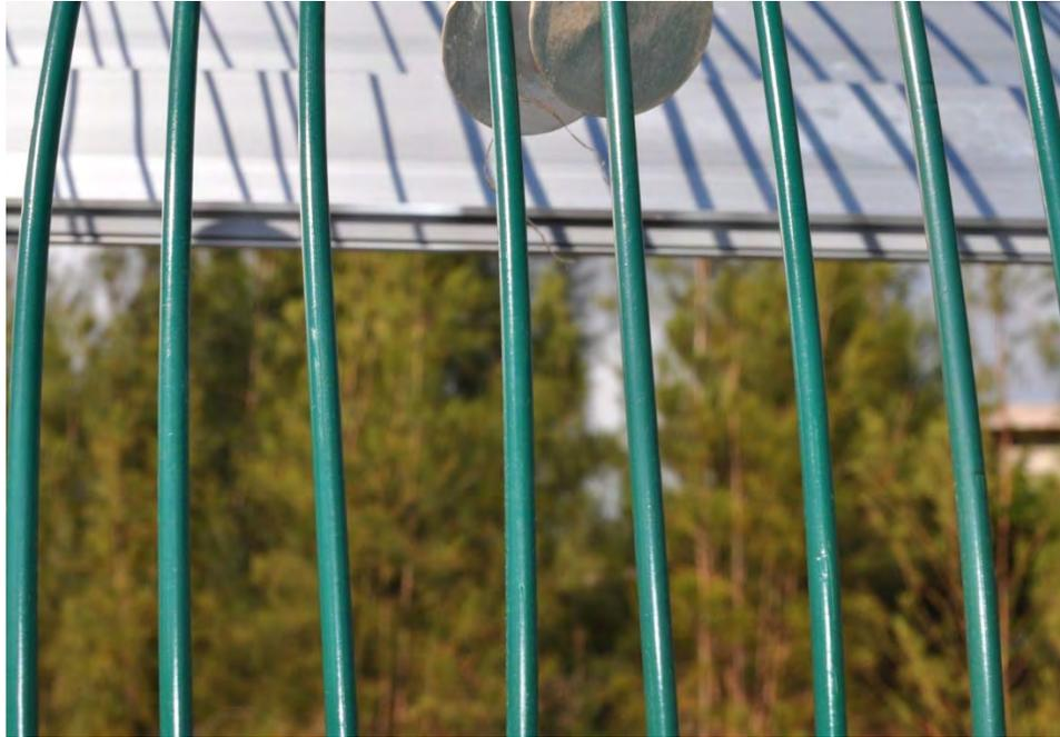
Figure B85. Standard PVC Coated Galvanized Wire Coupon
