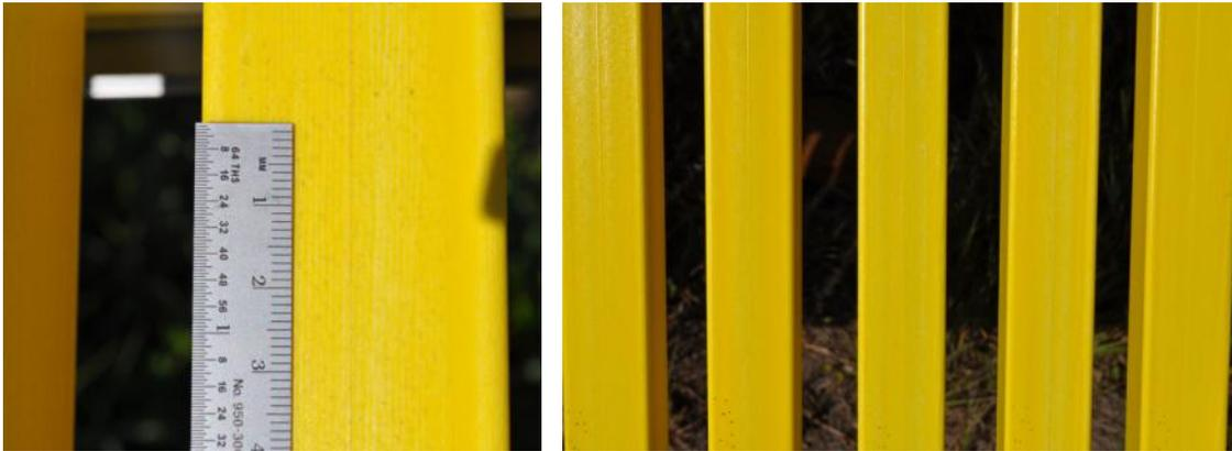
Figure 30. Coated steel railing coupon at FRF (left) and KTA (right) after 6 months of exposure.
