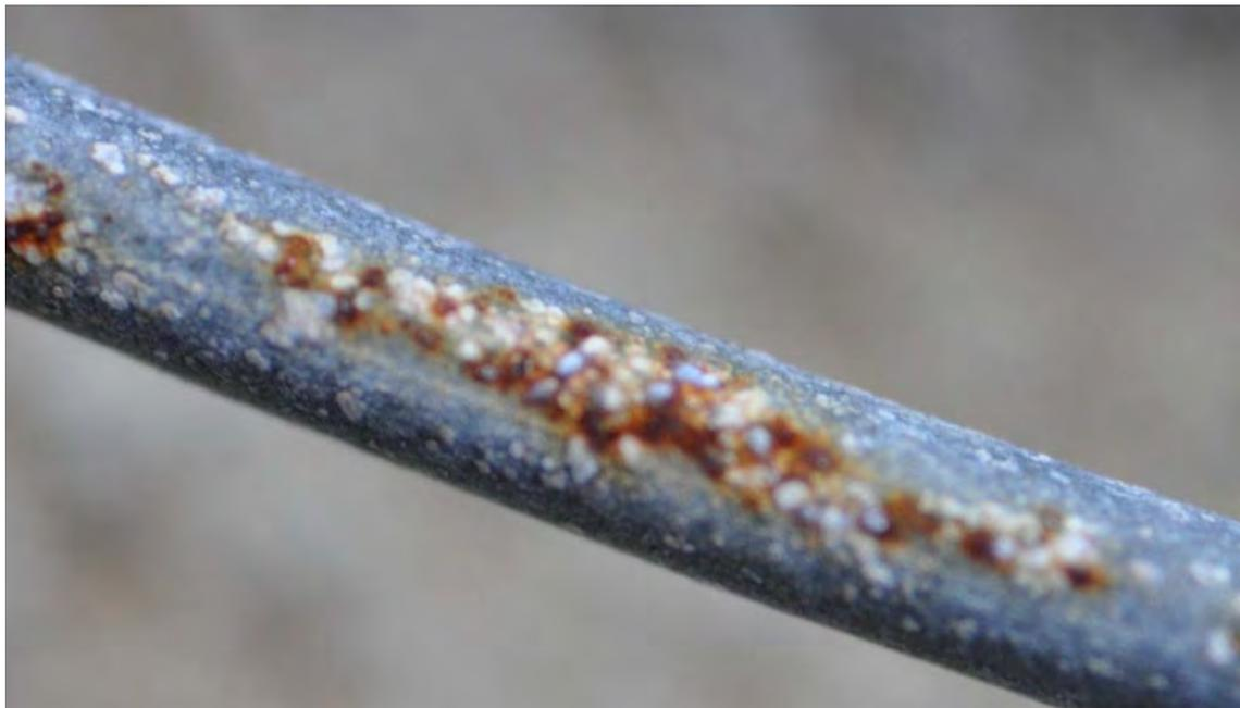
*Figure B126.* Standard Galvanized Wire Coupon
