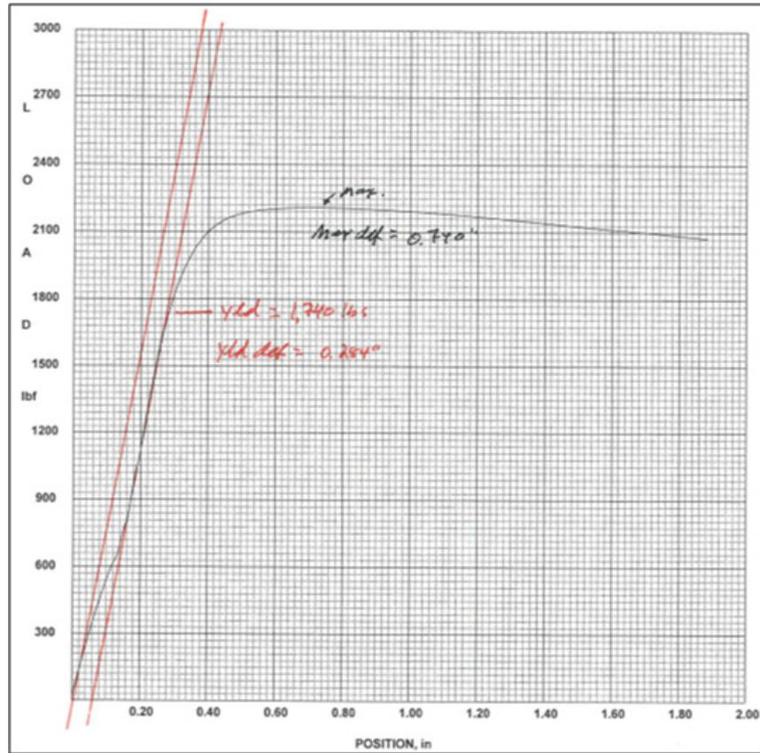
Figure 47. Cross sectional collapse of a stainless steel pipe under flexure testing.
