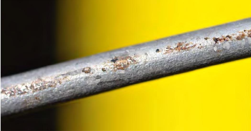
*Figure B177.* Aluminized Steel Wire Coupon
