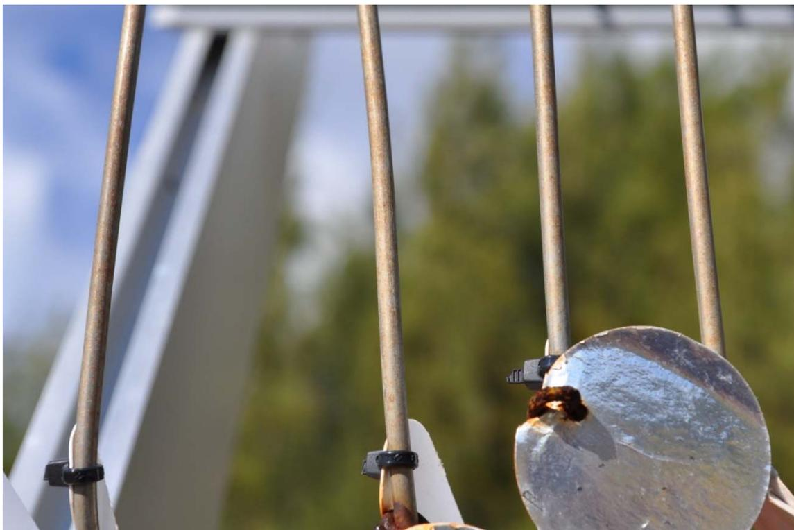
*Figure B94. Stainless Steel Wire Coupon*
