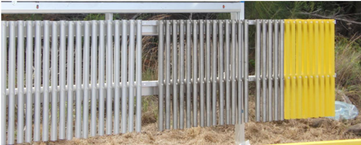
Figure 11. Railing and wire coupons installed on ASTM G7 exposure rack placed a 45 degree angle at KTA.
