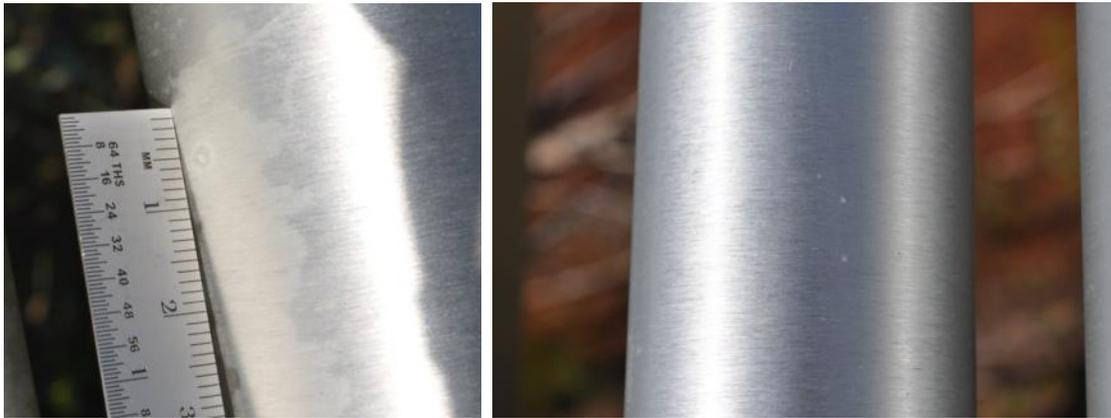
Figure 33. FRP railing coupon at FRF (left) and KTA (right) after 12 months of exposure.
