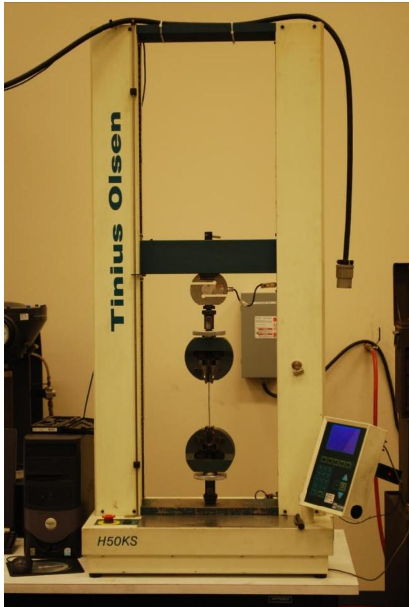
Figure 17. ASTM D790 flexure test of railing coupons after exposure.
