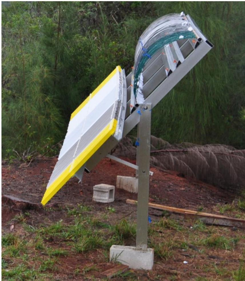
Figure 12. Railing and wire coupons on exposure rack placed at 45 degree angle at the FRF.
