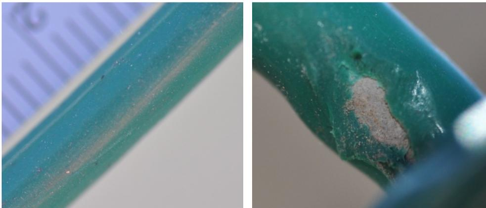
Figure A18. Aluminum 6061 T6 after 12 months exposure.
