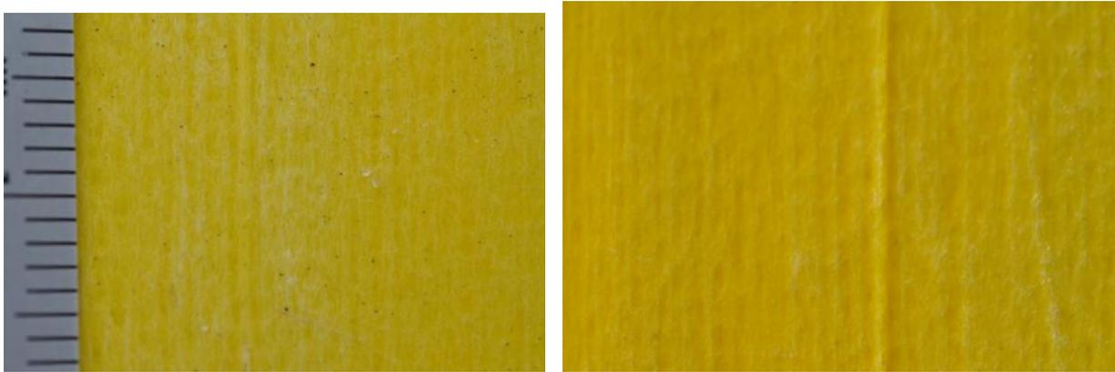
Figure 34. Coated steel railing coupon at FRF (left) and KTA (right) after 12 months of exposure.
