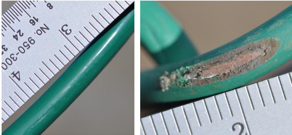
Figure A16. Galfan showing localized corrosion on 10% of its total surface after 12 months exposure.
