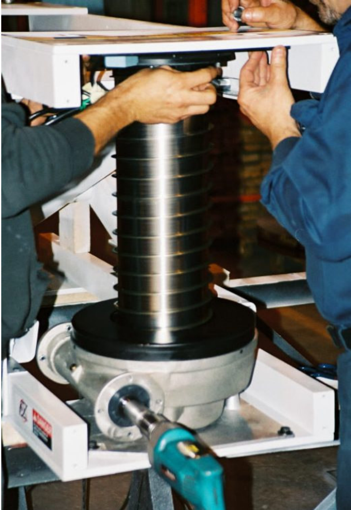
Six-Inch Spiralift Being Connected to Installation
