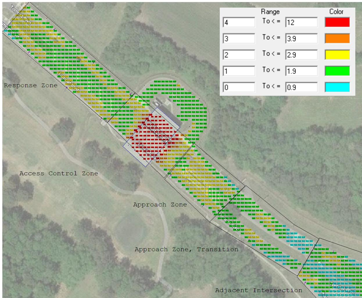
Figure 18 – Overall photometric plan of Gate B. Values shown in footcandles.
