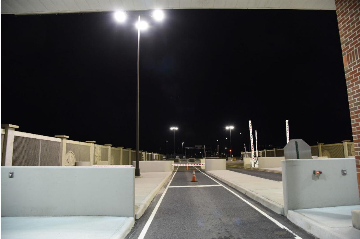
*Figure 15 – High glare luminaires directly in front of Security Personnel location in Access Control Zone*
