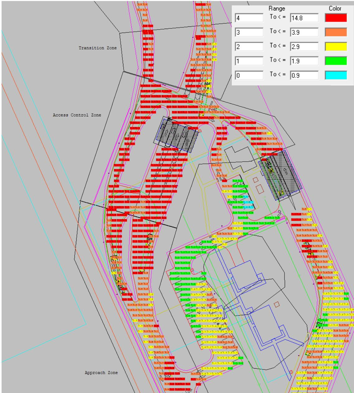
Figure 17 – Gate A Overall Photometric Plan. Values shown in footcandles
