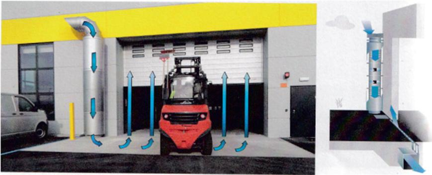
**Fig. 2.10** Schematic and an example of ACUHO air curtain application
