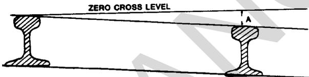
Figure 12-3. Crosslevel measurement.
