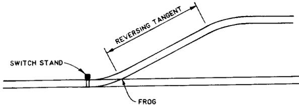
Figure 8-2. Reversing tangent length and switch stand placement.
