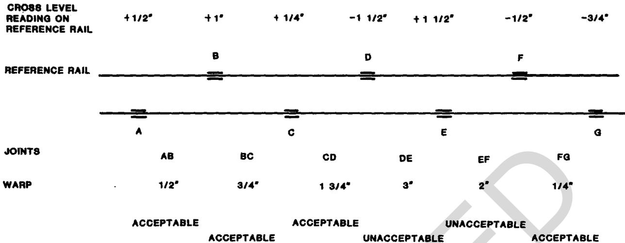
**NOTE: DISTANCE BETWEEN MEASUREMENTS IS 62 FEET OR LESS.
