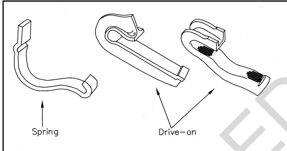
Figure 6-23. Rail Anchors
