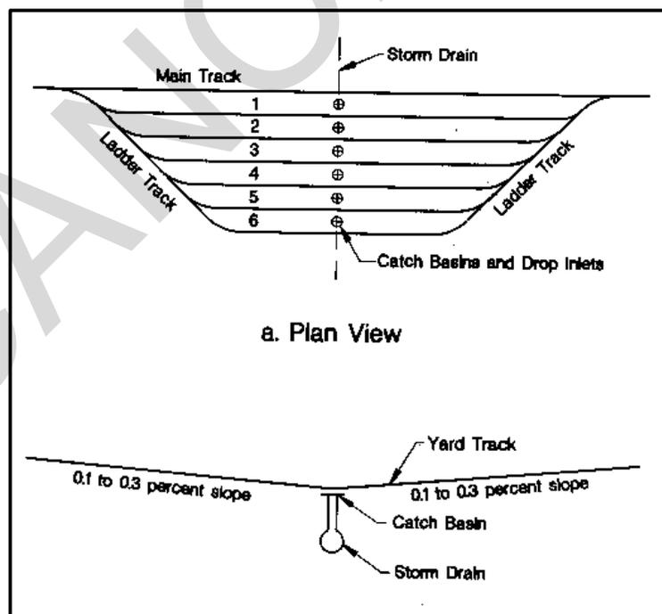
Figure 8-1. Typical Small Yard with Storm Drainage
