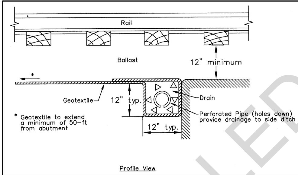
Figure 6-19. Geotextile Installation at a Bridge Abutment
