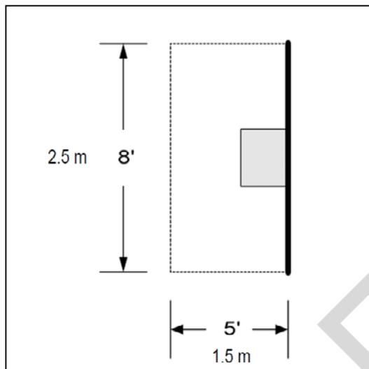
The workspace required around the cabinet/rack is still required even if the cabinet is mounted 6.5 feet (2.0 m) off the floor
