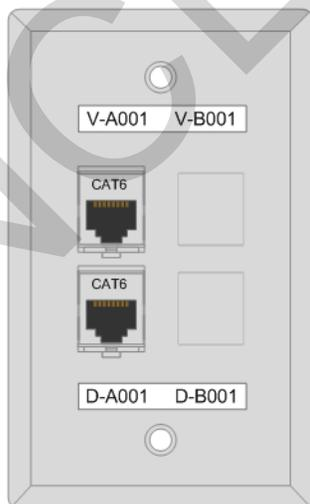
Figure 2-3 represents a single gang faceplate with two CAT6 modules, two blanks, and sample labeling. As the infrastructure converges to voice over internet protocol (VoIP), there will be no difference or distinction between voice or data modules.
