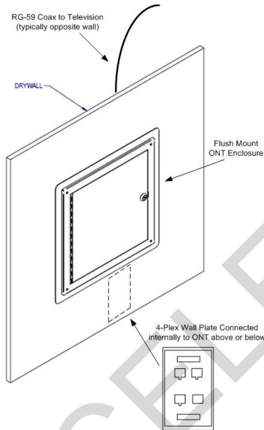
**Figure 6-2 Flush mounted ONT enclosure**
