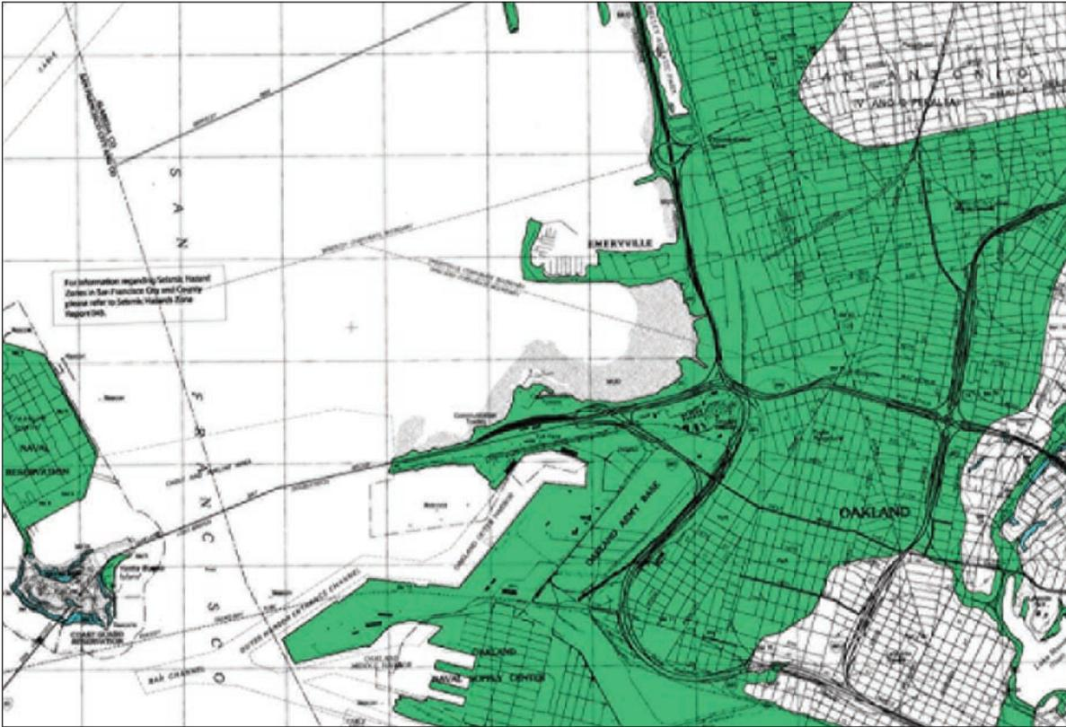
Figure 3-13: Liquefaction Hazard Zone Map for West Oakland and Emeryville.
