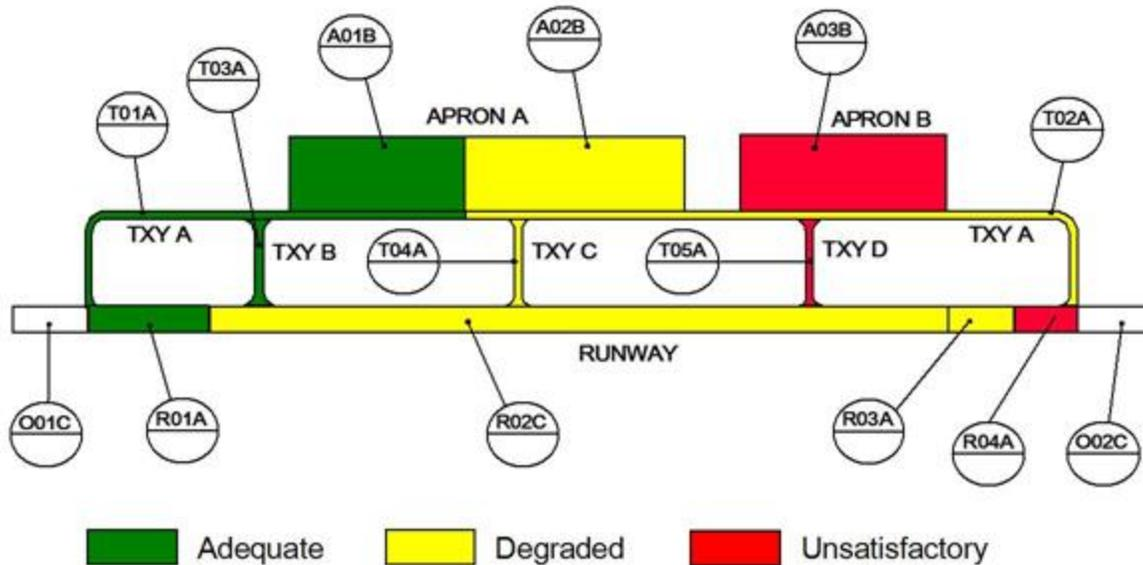
Figure 8.6. Sample Airfield Layout Plan Rated by Branch.
