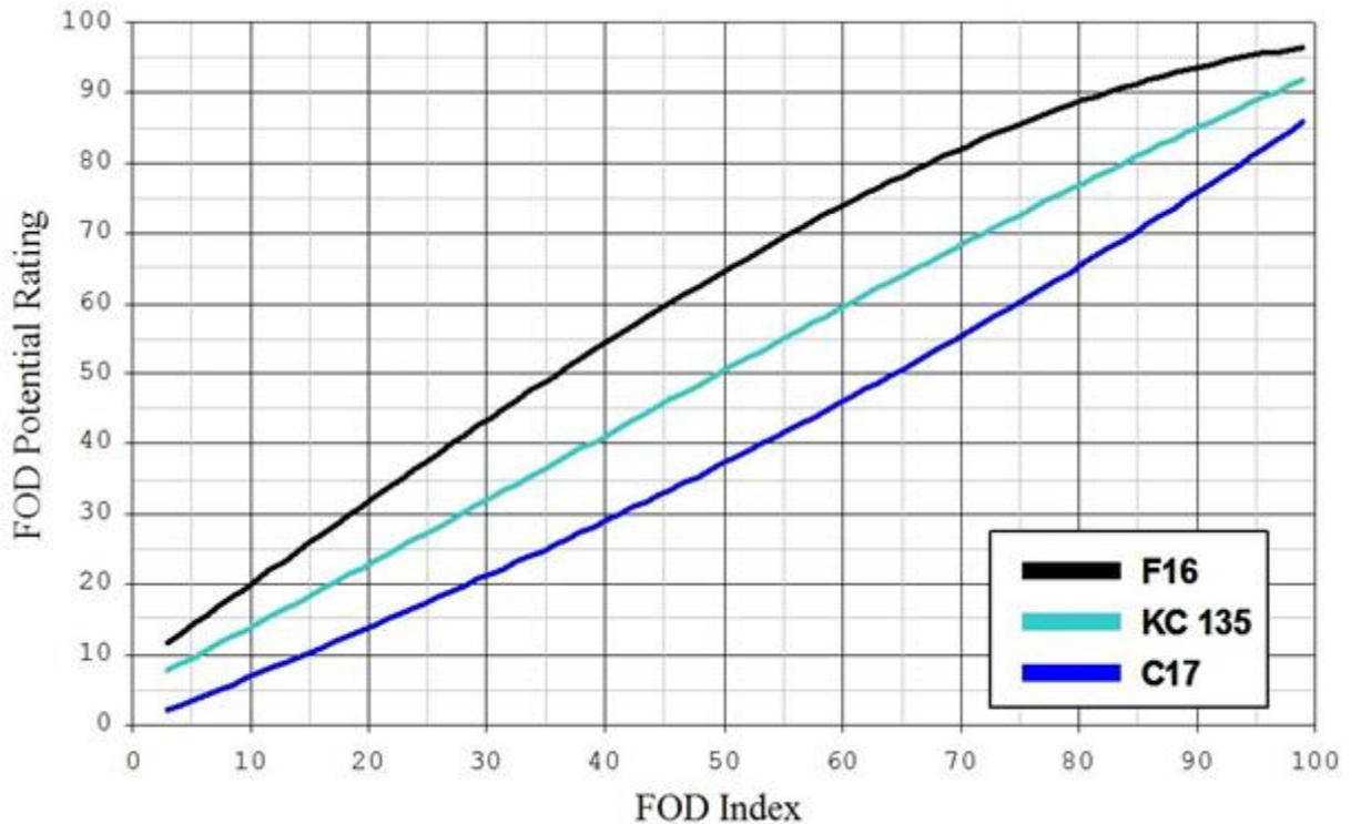
Figure 8.4. Relationships Between FOD Index and FOD Potential Rating for Concrete Payments.
