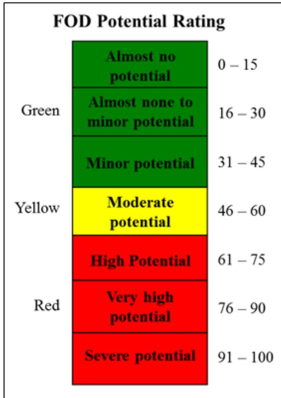
Figure 8.3. Relationships Between FOD Index and FOD Potential Rating for Asphalt Pavements.
